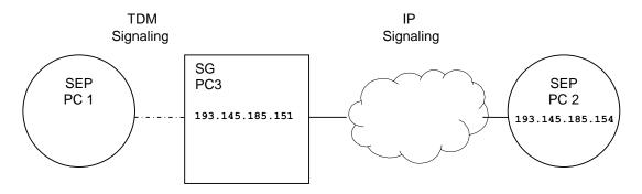
Figure 7 shows an example of a Signaling Gateway connected to a SEP on the TDM side and a SEP on the IP side.
